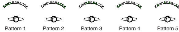
FIG. 1. (Color online) (A) Eleven loudspeakers evenly spaced in front of the listener ( 10^\circ separation) were used to present stimuli. (B) Maskers were presented from loudspeaker locations arranged into one of five masker patterns. Each pattern had four maskers, presented concurrently with the target.
